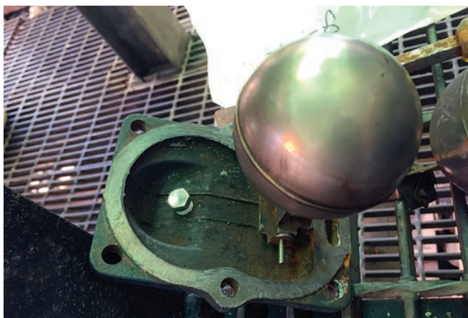
FIG. 4. Floater trap with thermostatic vent plugged.
