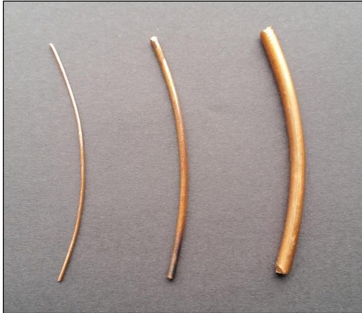
**Figure 5: Spacers for maintaining consistent HTC thickness.**
