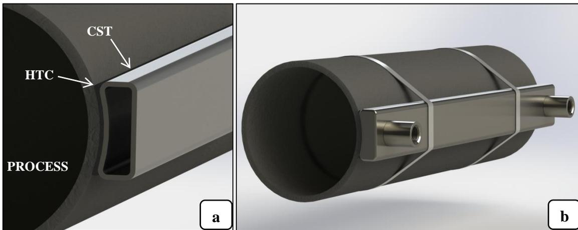
**Figure 1: a) View of CST profile mated to process pipe
