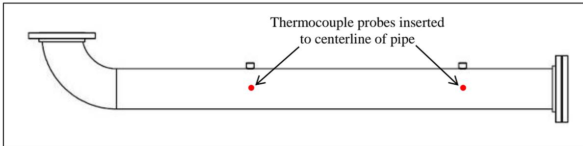
**Figure 6: Thermocouple probe measurement locations**
