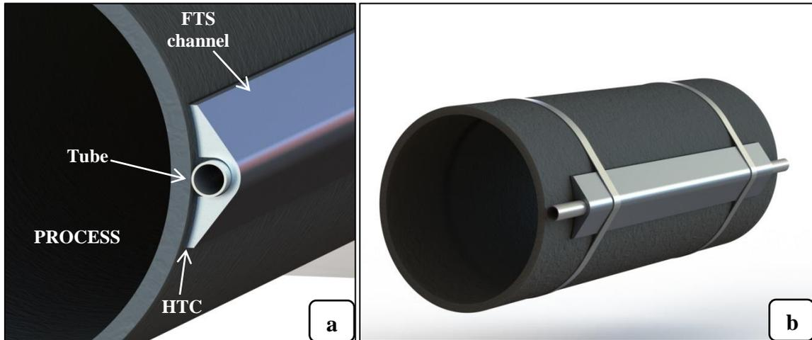
Figure 2: a) View of FTS profile mated to process pipe
