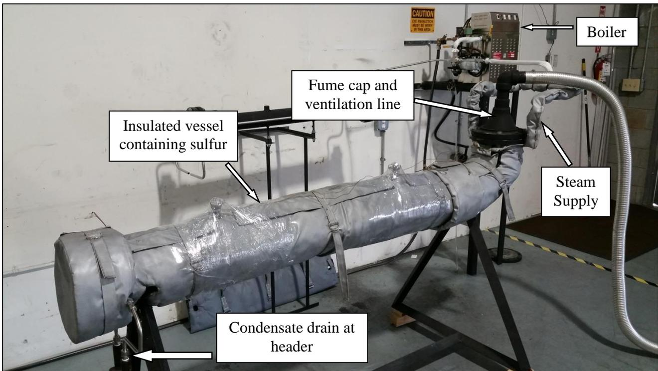
**Figure 4: Testing apparatus fabricated from 6-inch SCH. 40 carbon steel pipe**
