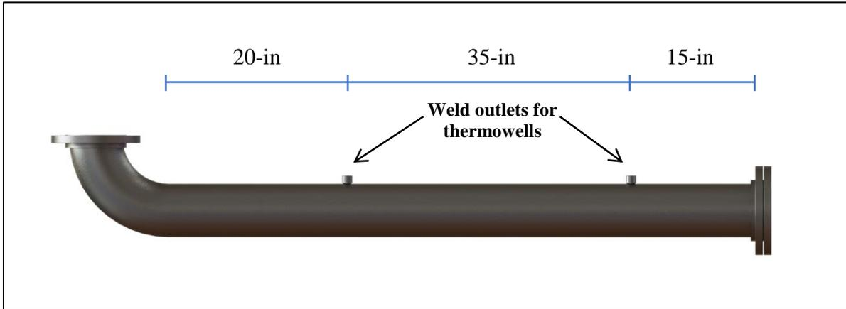
**Figure 3: Sulfur vessel for testing apparatus**
