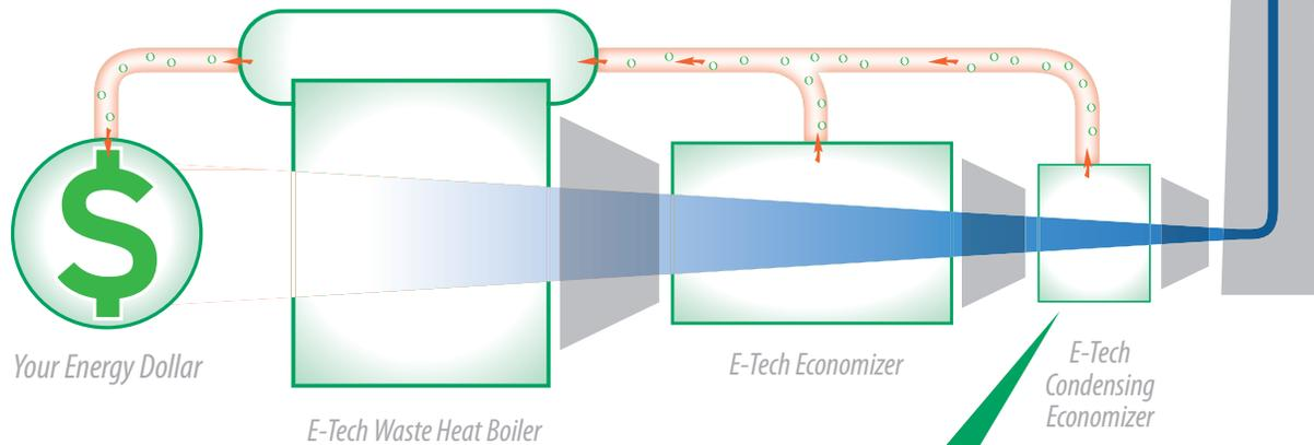
E-Tech **condensing economizers** yield extremely high efficiencies — upward of 96%. Their vapor-condensing environment presents an ideal heat recovery solution for industries that use non-sulfur bearing fuels, whose acidic byproducts can corrode most carbon and alloy materials.
