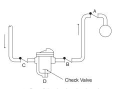
Fig. 1-8. Possible check valve locations.
