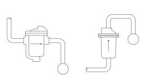
**Fig. 2-5.** Traps installed with short, well pitched discharge lines to prevent freezeups.
