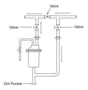
**Fig. 1-6.** Bypass hook-up for No. 211-216 & 411 traps.
