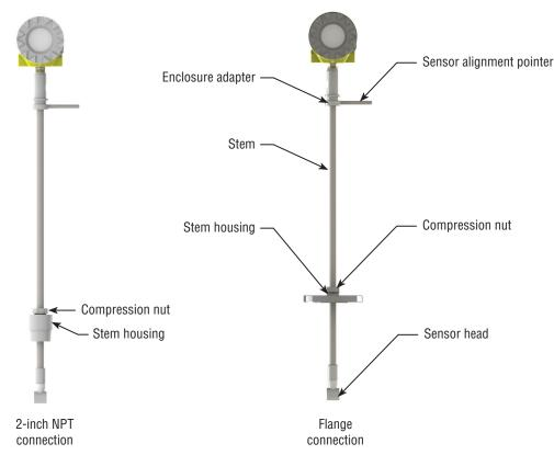
Figure 2-7. Flow Meter with Compression Type Fitting
