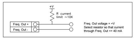
Figure 2-19. Isolated Frequency Output Using External Power Supply
