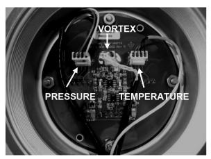
Figure 5-2. Remote Feed Through Board Sensor Connections
