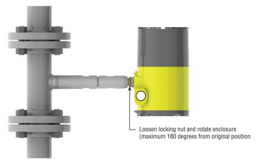
Figure 2-13. Enclosure Viewing Adjustment
