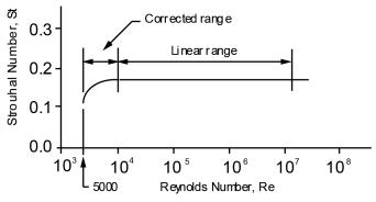
Figure 1-3. Reynolds Number Range for the AVF and AVI vortex meters
