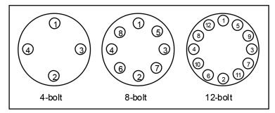
Figure 2-2. Flange Bolt Torquing Sequence
