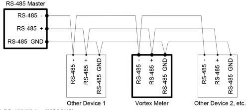
Figure 4-4.RS-485 Wiring (MODBUS)
