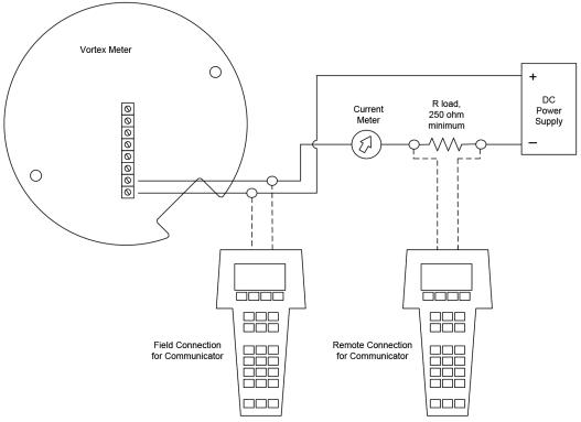
Figure 4-1.Loop Powered Meter Wiring (HART)
