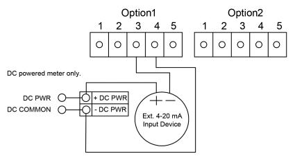
Figure 2-45. External 4-20 mA Input Wiring - DC Powered Meter
