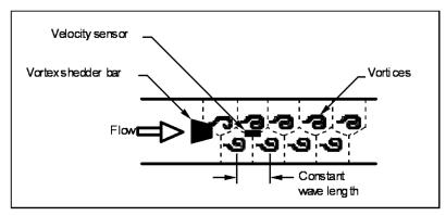
Figure 1-2. Measurement Principle of Vortex Flow Meters
