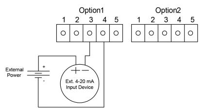
Figure 2-44. External 4-20 mA Input Wiring - External Power Supply
