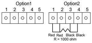
Figure 2-43.Optional Energy EMS RTD Input Wiring
