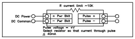
Figure 2-18. Non-Isolated Pulse Output Using External Power Supply
