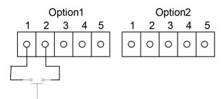
Figure 2-47. Optional Contact Closure Input Wiring
