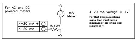
Figure 2-30. Isolated 4–20 mA Output Using External Power Supply
