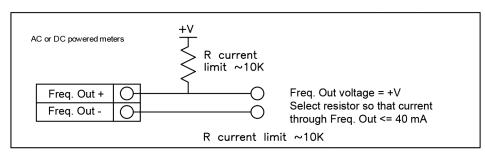
Figure 2-33. Isolated Frequency Output Using External Power Supply
