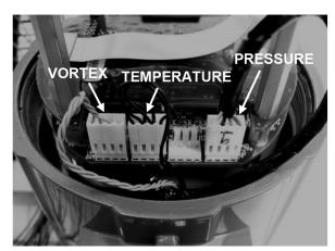
Figure 5-1.Electronics Stack Sensor Connections
