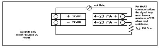
Figure 2-32. Isolated 4–20 mA Output Using Meter Provided Power Supply
