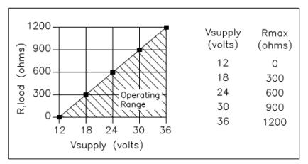
Figure 2-16. Load Resistance Versus Input Voltage
