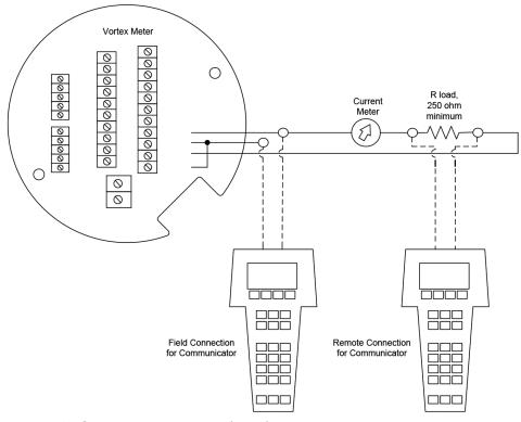
Figure 4-3.AC Powered Meter Wiring (HART)
