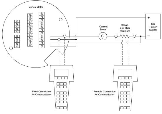
Figure 4-2.DC Powered Meter Wiring (HART)
