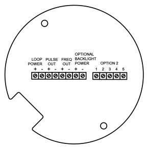
Figure 2-14. Loop Power Wiring Terminals
