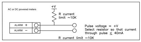
Figure 2-39. Isolated Alarm Output Using External Power Supply
