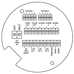
Figure 2-25. AC Wiring Terminals
