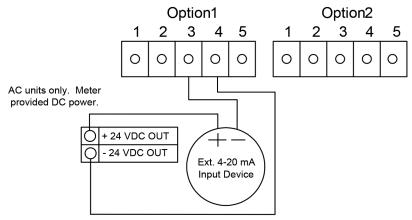
Figure 2-46. External 4-20 mA Input Wiring - AC Powered Meter
