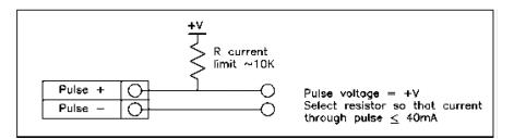
Figure 2-17. Isolated Pulse Output Using External Power Supply
