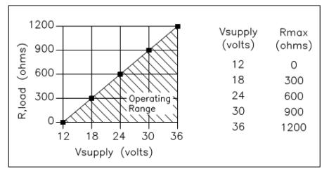
Figure 2-29. Load Resistance Versus Input Voltage
