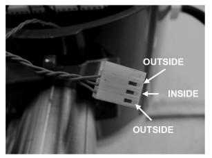
Figure 5-3.Vortex Sensor Connector
