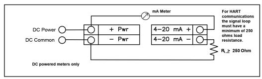
Figure 2-31. Non-Isolated 4–20 mA Output Using Meter Input Power Supply
