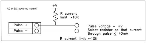
Figure 2-36. Isolated Pulse Output Using External Power Supply
