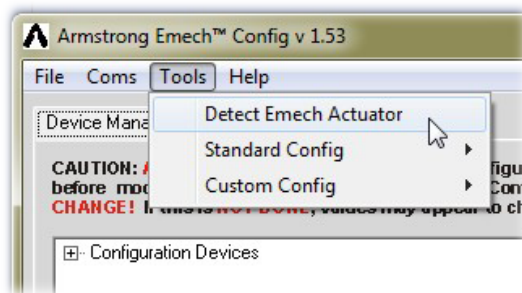
Figure 5.2: Detecting an Emech actuator if unsure of which COM port to use.
