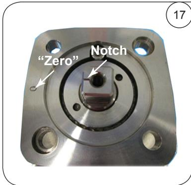
17 Insert the locking screw after applying a thread locking adhesive (Image 17). Tighten the locking screw as per the torque values given in table 4.1.
