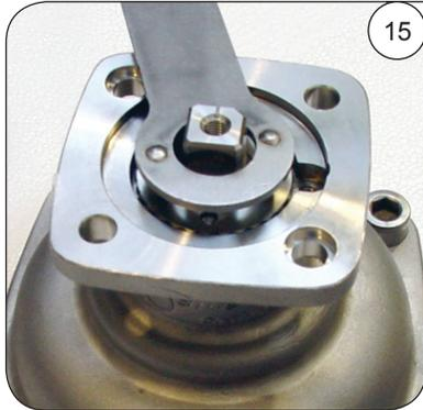
15 With the gland wench provided, screw the gland nut down until it bottoms out. Do not over-tighten! (Image 15).
