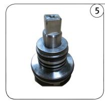
In either situation, the spindle will need to have two O-rings and two wear rings removed (Image 5).
