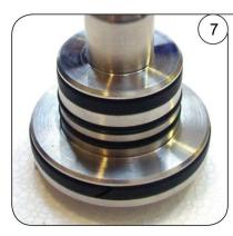
Apply a light even coat of grease to the spindle bearing surfaces and the O-rings (Image 7).
