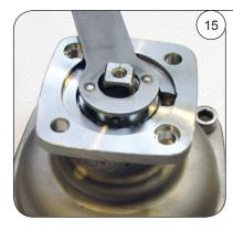
With the gland wench provided, screw the gland nut down until it bottoms out. Do not over-tighten! (Image 15).
