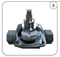
NOTE: The spindle should be tight fitting. If the spindle does not sit flat on top of the disc, clean lugs. If the spindle still does not sit flat, file the lugs.
