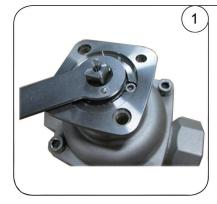
Replace the pins if they are damaged. Before assembling/re-assembling the valve, make sure hands are free of dirt and grease and the valve is clean.
