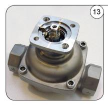
Rotate the spindle one full rotation. The movement should be smooth and even with no variation in torque (Image 13).
