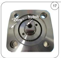
Insert the locking screw after applying a thread locking adhesive (Image 17). Tighten the locking screw as per the torque values given in table 4.1.
