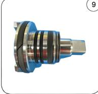
Lightly grease both sides of the thrust washer and place on the spindle. Place on the needle roller bearing (Image 9) and apply grease (approx 60% of the void space). Lightly grease both sides of the second thrust washer and place on the bearing.
