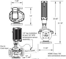
NOTE: The assembly can be changed to have either port A or port B as hot or cold
