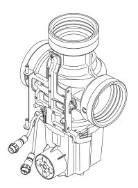
Attach the Electronics Module and secure using the circlip supplied.
