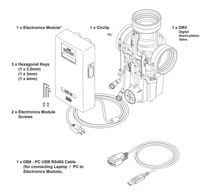
\*2 x CR - P2 6V Batteries fitted as supplied. USB Driver and The Brain® DRV80 Control Software are available to download from website, www.armstronginternational.com/brain
