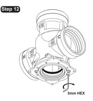
Use one of the 3mm Hex screws to assist in refitting the cartridge. Remove the screw when the cartridge is inserted fully.
