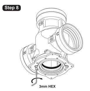
Use one of the 3mm Hex screws to assist in removing the cartridge.
