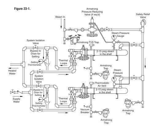
**NOTE:** Depending on capacity requirements a parallel water heater installation may also require (2) two PRV's in parallel. Single wall installation shown - Double wall would be similar. See your Armstrong Representative for proper reducing valve application.
