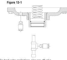
**Note:** For hard water applications, pipe pop-off valve into dirt leg.
