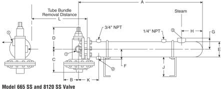
**Note:** Heavy duty 5/8" tubes of 16 gauge 316L stainless steel ensure long life and maintainability backed up by a 10-year tube bundle warranty against workmanship and material defects.
