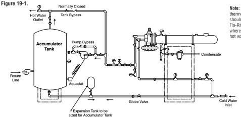
Note: Position of system thermometer. Thermometers should not be placed between Flo-Rite-Temp and "T" fitting where3-Way valve ties back into hot water outlet.
