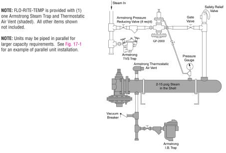
The unit includes the mixing valve mounted to the heat exchanger, channel iron and U-bolts mounted, thermostatic air vent installed on the heat exchanger, a water pressure pop off valve integral to the unit control valve and a separate Armstrong Inverted Bucket Steam Trap.
