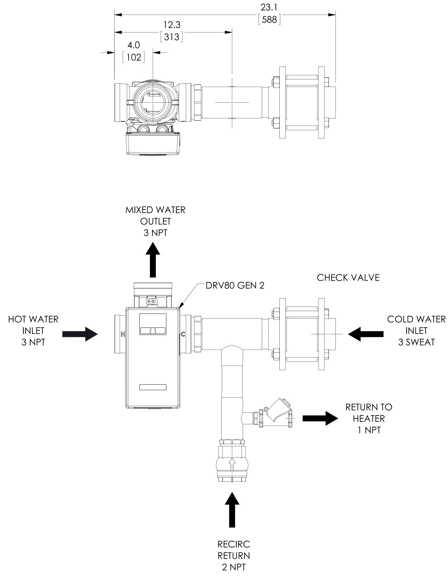
NOTE: ALL VALVES AND FITTINGS IN THIS ASSEMBLY CONTAIN LESS THAN 0.25% LEAD BY WEIGHTED AVERAGE
