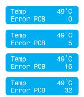
Indicates the PCB has failed, replace the PCB.
