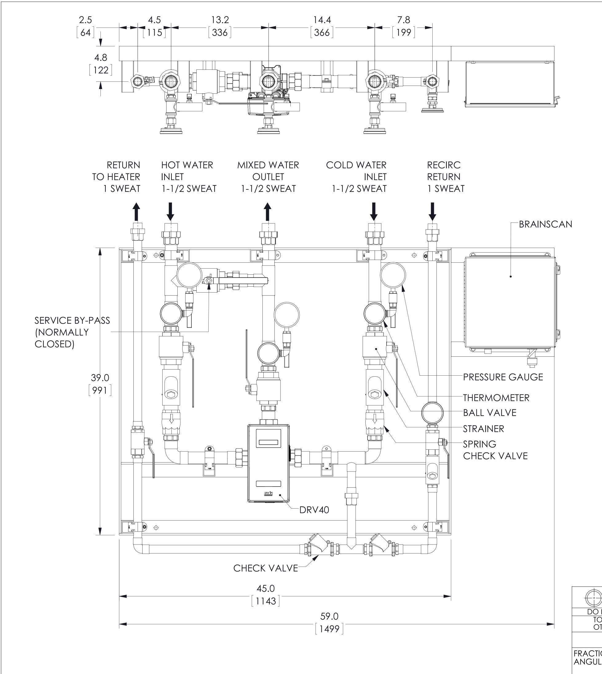
NOTE: ALL VALVES AND FITTINGS IN THIS ASSEMBLY CONTAIN LESS THAN 0.25% LEAD BY WEIGHTED AVERAGE
