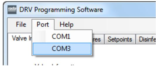
Locate the DRV40 by selecting the correct **COM Port**. The COM Port can be confirmed using the **Device Manager** utility within the Microsoft Windows OS.
