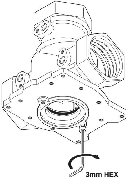
*Use one of the 3mm Hex screws to assist in removing the cartridge.*
