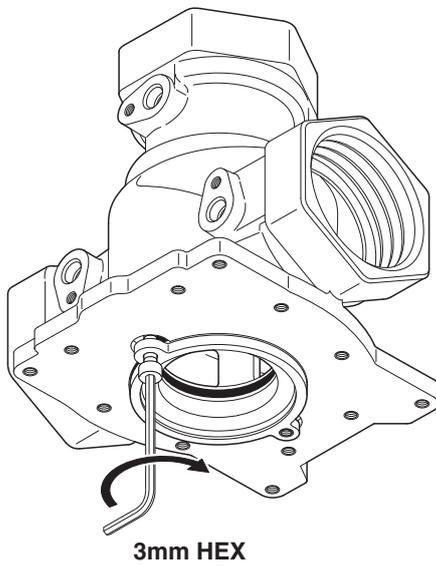
*Use one of the 3mm Hex screws to assist in refitting the cartridge.
