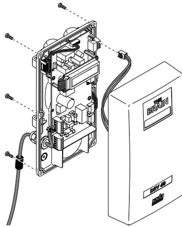
Isolate power to the DRV40 **before** disconnecting and removing the Electronics Module, see pages 43-46. Adjust the brightness setting on the PCB and reconnect the Electronics Module.
