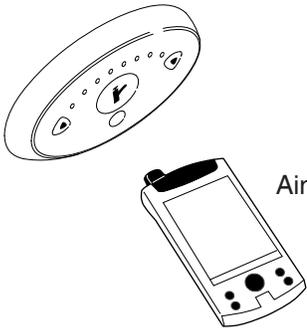
Aim the Programmer at the Control Panel and tap **“Read Log”**.
