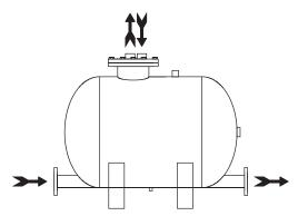
**Note:** Although the maximum operating pressure is 150 psig (10.34 bar), Armstrong Fluid Handling recommends that the motive pressure be set to 30 psig (2.07 bar) above the back pressure. This will provide optimum performance and reduce venting time between cycles.
