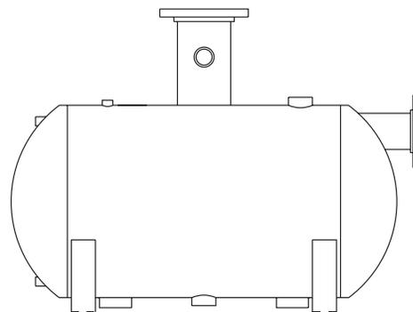
If the flash tank is held at atmospheric pressure, the use of a steam trap on the discharge line would not be necessary since the flash steam is being vented to atmosphere. The condensate, in this case, would be drained by gravity to a vented receiver which would be placed below the level of the flash tank.
