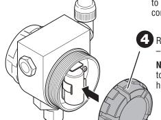
Reinstall back housing cap – torque 25 ft-lb (34 N-m).
