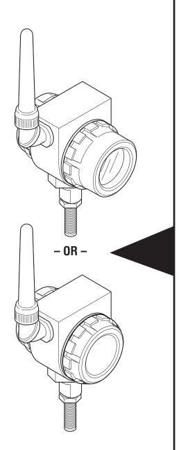
Remove front housing cap. **Programming Pins** (with display) (without display)
