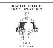
Oil floats to top, water is discharged from bottom. Body will fill with oil. If oil is heavy, trap is likely to stop operating.
