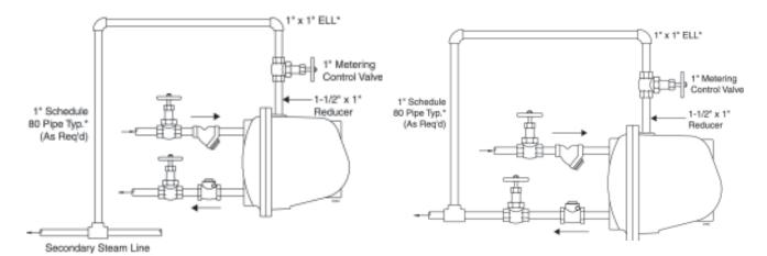
**Figure 3**Piping arrangement when secondary steam is collected and reused in heat transfer equipment.
