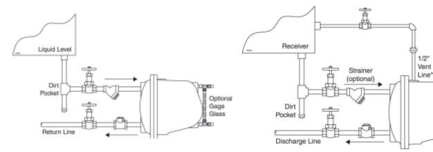
**Figure 1**"L" and "LS" Steam Trap or Condensate Controller.
