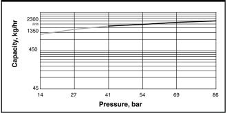
Note: Cold water capacity for start-up loads only. When superheat present, there will be minimal condensate. Grey curve indicates that trap can not be used in this area.
