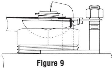
A stop lock nut, as shown in Fig. 9 must be installed in traps No. 216, 316, 416, 816 with 1-1/16" Orifice.
