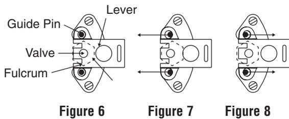
9. Hook bucket to valve lever and remove cap from vise. The trap is now ready for assembly.
